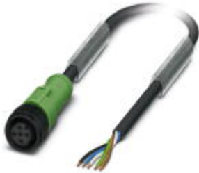
Sensor/Actuator cable, 5-position, PUR halogen-free, Black-gray RAL 7021, Free cable end, on Socket straight M12, A-coded, Cable length: 1.5 m, with plastic knurl
